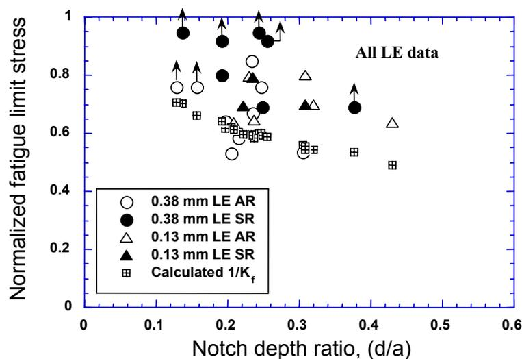
**Figure 3:** Effect of the notch depth ratio on the normalized fatigue limit stress for ballistically impacted 0.38 mm leading edge radius samples.
