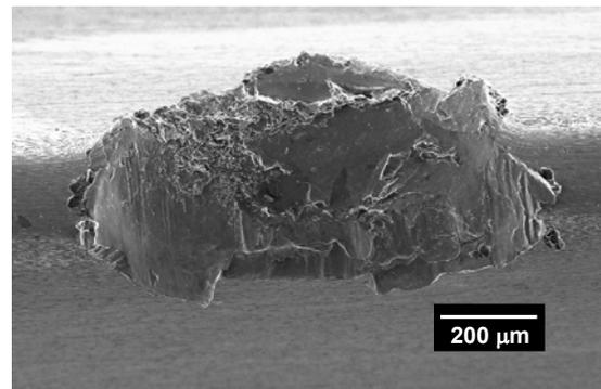
**Figure 1b:** Head-on view of a 30° ballistic impact FOD site for a 0.38 mm leading edge radius sample exhibiting a larger loss of material.
