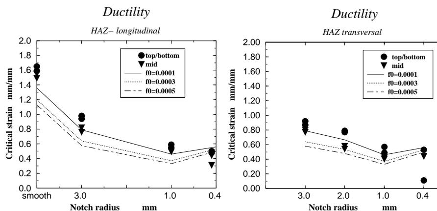
**Figure 5:** Ductility diagrams for HAZ. Longitudinal direction and cluster model (left), transversal direction and cluster model (right).
