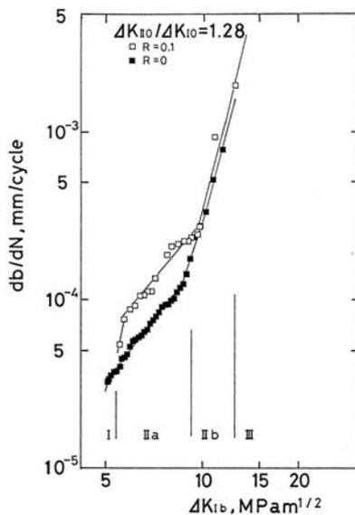
Figure 2: Characteristics of the  $db/dN$  under mixed-mode conditions.
