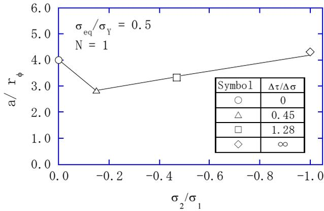
**Figure 6:** Effect of mixed-mode loading on the length,  $r_\phi$ , of the plastic zone along the direction of the main crack growth.
