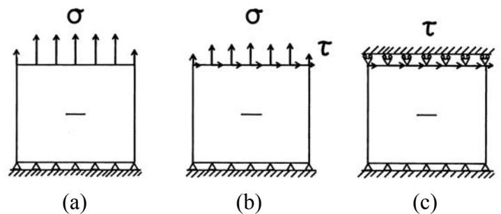
Figure 4: Model for mode I, mixed-mode and mode II conditions for the elastic-plastic FE analyses :
