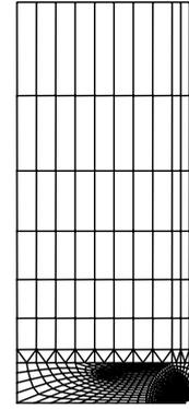
Figure 2: FE mesh of the narrow notch model
