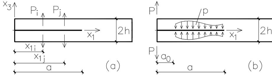
Figure 1: Schematic of the DCB specimen under different loading conditions.
