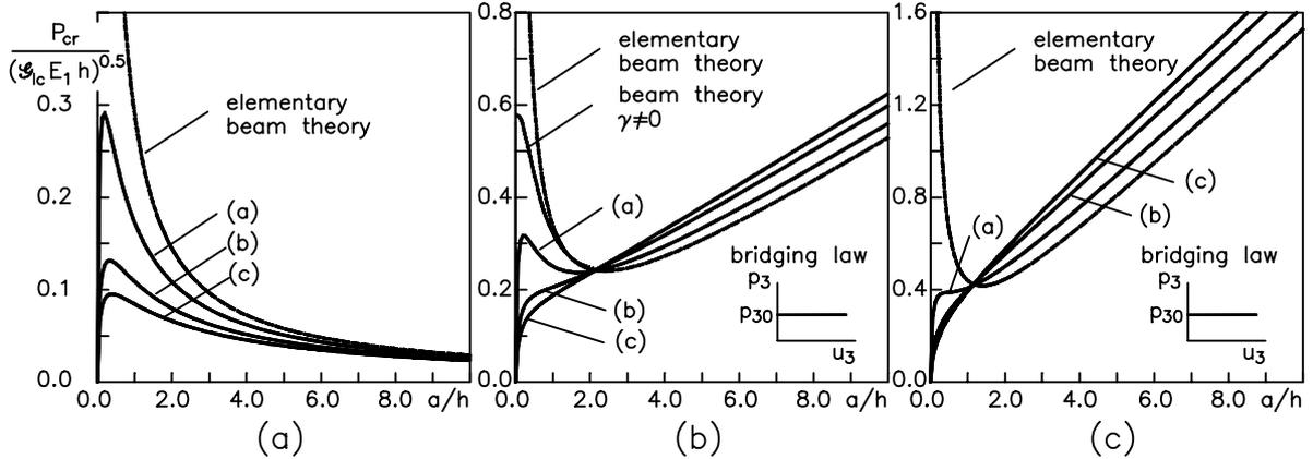
Figure 2: Dimensionless critical load versus normalized crack length in orthotropic DCB specimens. (a) No bridging. (b) Bridging tractions  $p_3 = 0.1 \sqrt{G_{Ic} E_1 / h}$ . (c) Bridging tractions  $p_3 = 0.3 \sqrt{G_{Ic} E_1 / h}$ .
