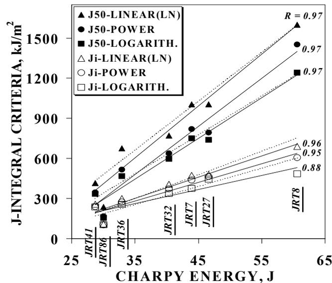
**Figure 5:**  $J_i$  and  $J_{50}$  criteria for all test pieces, as predicted by the LN technique. Dashed lines correspond to UEC results under the same testing conditions.  $R$  is the determination coefficient of the LN straight lines.
