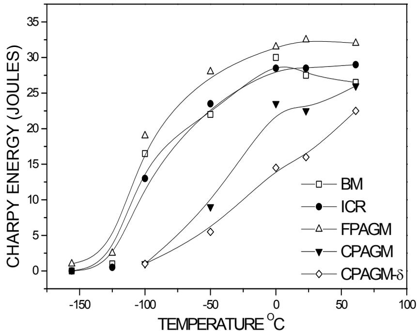
**Figure 1:** Charpy test results for simulated HAZ samples
