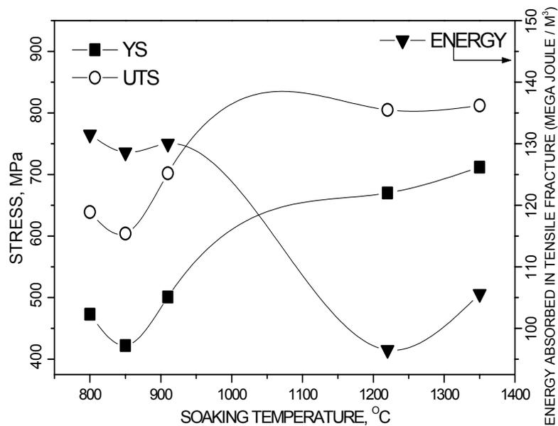
**Figure 3:** Tensile test results of simulated HAZ samples
