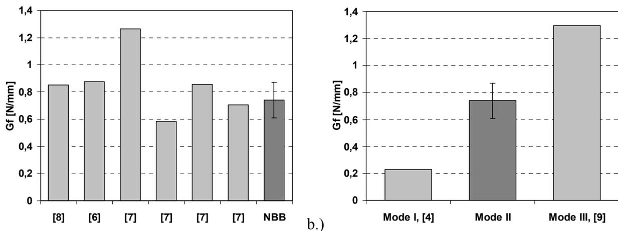
**Figure 4:** (a) Comparison of overall mean specific fracture energies ( $G_f^{II}$ ) obtained by NBB specimens with values for spruce wood reported from literature [numbers]. (b) Mode II specific fracture energy ( $G_f^{II}$ ) related to mode I and mode III loading conditions
