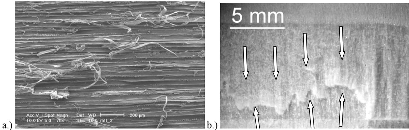
**Figure 4:** (a) ESEM image of mode II fracture surface of spruce wood; (b) Light microscopical image of mode II fracture surface. The arrows mark contrary crack propagation directions in different fracture planes.
