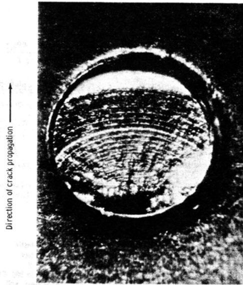
Figure 6. - Fracture surface of 1/4 inch diameter copper specimen showing striations. N_f = 104 cycles.
