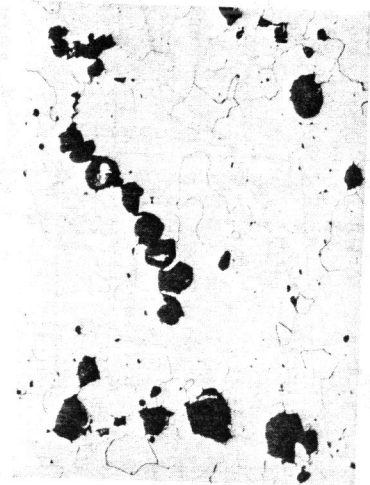
FIG. 7. TYPICAL FISSURES WHICH RESULTED FROM JOINING OF GAS BUBBLES IN ANNEALED CARBON-STEEL CAUSED BY 245 HOURS OF EXPOSURE TO 63 ATM HYDROGEN AT 540° C. 76X
