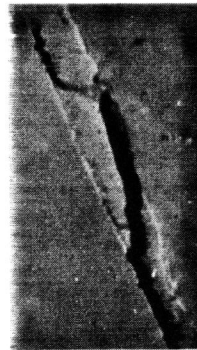
Fig. 8 Cracks associated with a twin. Original surface. P4, -160^{\circ}\text{C} . 370X.
