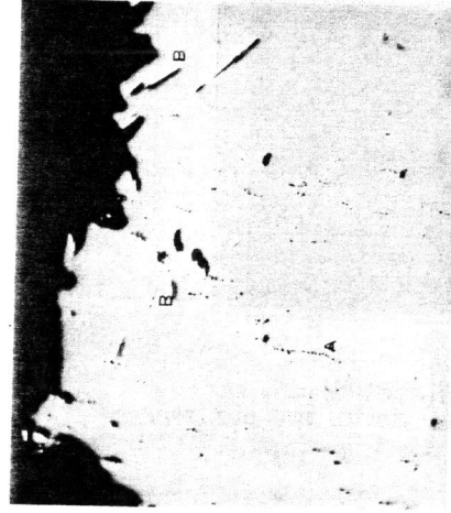
(a) Voids in neck of F4 specimen at fracture. 32.3% reduction in area. Note cracked carbides at (A) and cleavage cracks at (B). Fracture about 10% fibrous. Tested at -90°C.
