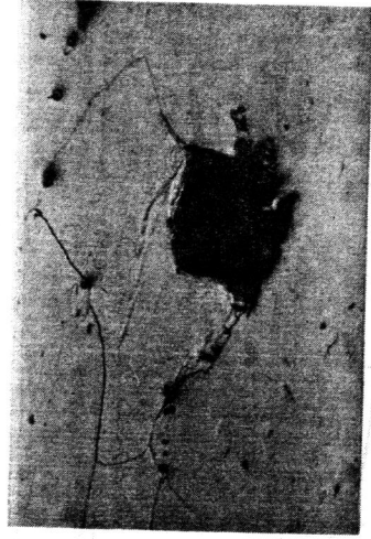
(b) Large void from cracked carbide in neck of F4 specimen near fracture. 70.0% reduction in area. Tested at -70°C.
