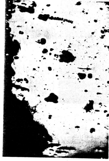
(c) Voids in neck of F4 specimen at fracture. 70.0% reduction in area. Note increase in size of holes from cracked carbides as strain in the neck increases. Fracture about 95% fibrous. Tested at -70°C.
