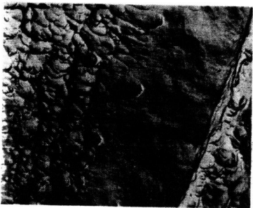
Figure 8 - PLASTIC FRACTURE - TEAR MODE - Elongated dimples resulting from a tear plastic fracture in a 4340 steel. See Sketch 5c. 3000X
