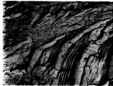
Figure 22 - FATIGUE FRACTURE - Ductile and brittle striations in a 7178 aluminum alloy occur in adjacent areas, but only the ductile striations are clearly defined.
