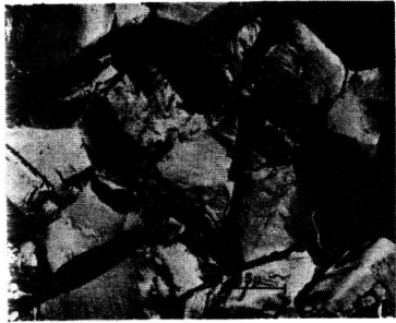
Figure 14 - INTERGRANULAR FRACTURE - Brittle intergranular fracture in a 70-30 brass. This fracture is the result of a slow crack propagation under cyclic load in a centrally notched panel of brass. 3000X
