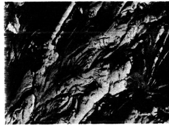
Figure 4 - CLEAVAGE FRACTURE - Cleavage fracture in a Tm molybdenum alloy. The large cleavage "feathers" are made up of many cleavage facets. Extensive tear takes place between the large regions of cleavage. 3800X
