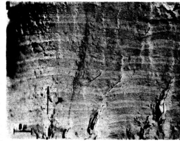
Figure 25 - FATIGUE FRACTURE - Three distinct growth bands are apparent in the fracture topography of this spectrum loaded 7178 aluminum alloy. Loading in this spectrum was divided into three general load levels. Even though striations are not clearly defined in each area, some growth did occur.
