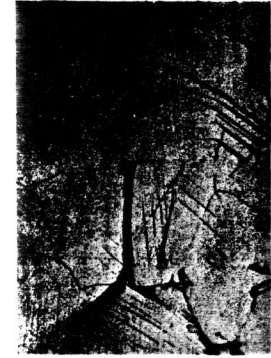
Figure 3. Microcrack in ferrite tested in tension at -140^{\circ} C 170X
