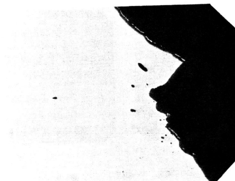
Figure 3. Longitudinal section through fractured superpurity aluminium deformed at 85 °K. Fine grained. 40X
