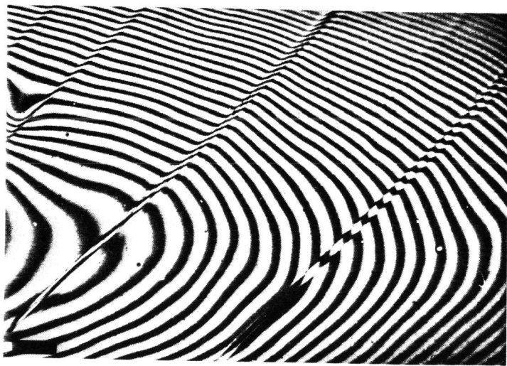
Fig.8 as fig.7, only for Cu 6.5% Ge crystal, cycled at \tau = 4.7 \text{ kg mm}^{-2} .
