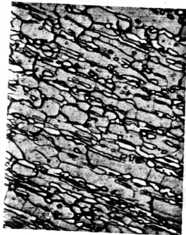
Fig. 2 Photomicrograph of ductile 40% Pt - 60% Au alloy annealed 97 hours at 980°C. Magnification 280X
