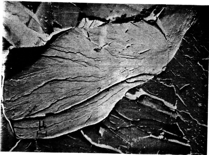
Figure 9 - Low-carbon steel. Crossing of grain boundary; re-nucleation of crack at a single point from which the crack fans out across the grain.
