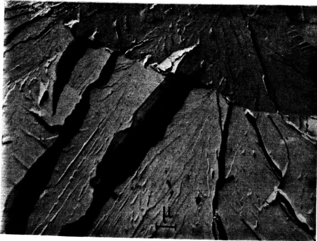
Figure 8 - Low-carbon steel. Crossing of grain boundary : re-nucleation of crack at several different points. The direction of crack propagation is from the upper right towards the lower left corner of the micrograph.
