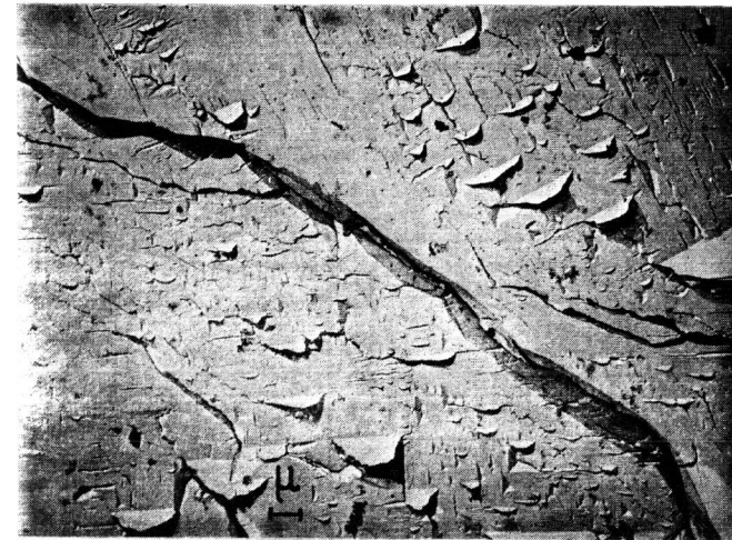
Figure 1 - Low carbon steel. Impact cleavage fracture at -196^{\circ}\text{C} . "Tongues".
