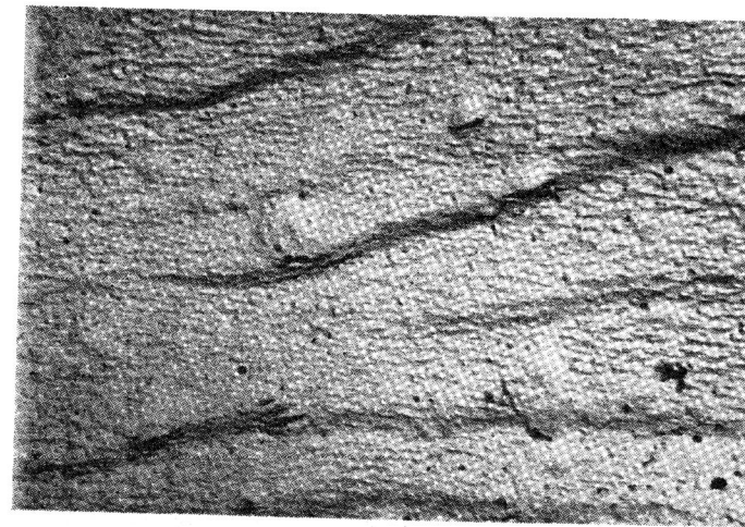
Fig. 21. Electron micrograph of the same surface shown in Fig. 20. The engraved appearance of the surface is due to electropolishing.
