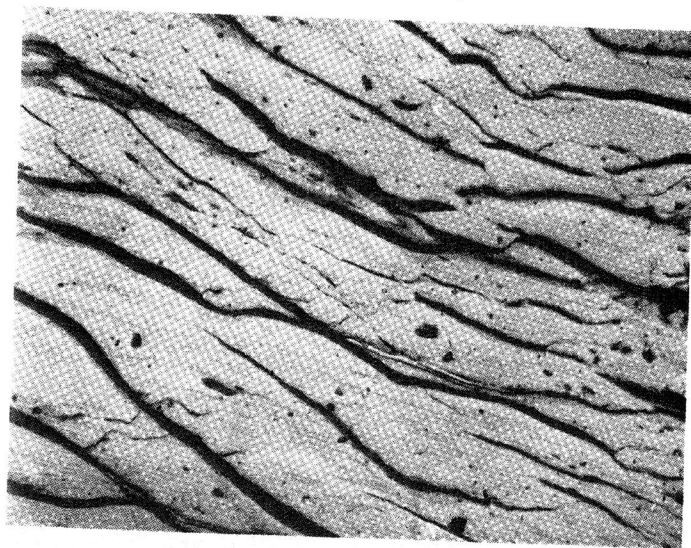
Fig. 26. Electron micrograph of the surface of a mild-steel sheet after 1 bending cycle, repolishing, and bending again.
