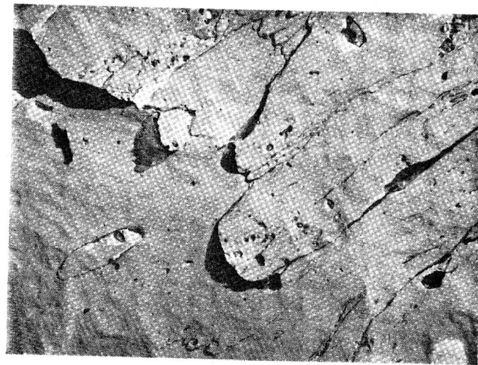
Fig. 13. Microfractograph of a "decohesion along glide plane" with very elongated dimples. Same rupture surface as in Fig. 9.
