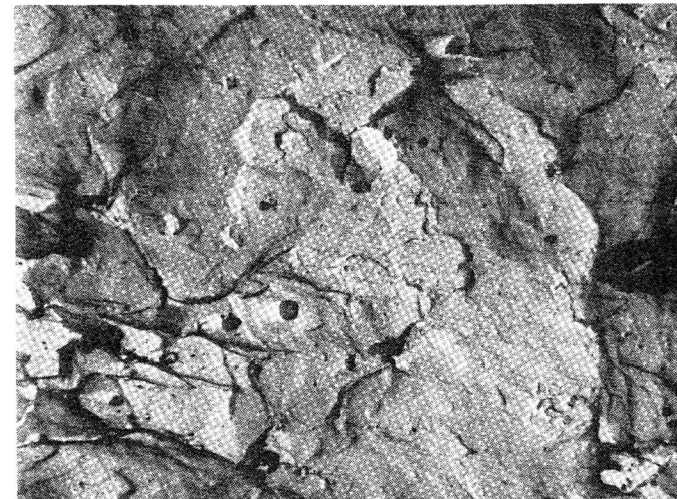
Fig. 19. Microfractograph of a fatigue rupture surface of mild steel after 15% prestrain in tension (rupture in 0.62 \times 10^6 cycles, direct stress 10 \pm 16 \text{ kg/mm}^2 ).
