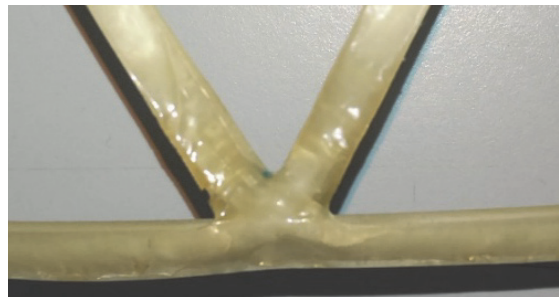
Figure 11: Defect absence in the circumferential head trajectory.
