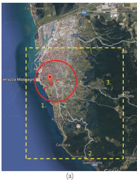
Figure 9: Identification of study cases. The bridge 1 is localized in the urban area while the bridges 2 and 3 in a suburban one. The circle highlights the flooded area where the Rio Maggiore overflowed (a). Catching basins related to sections 1, 2 and 3 (b).
