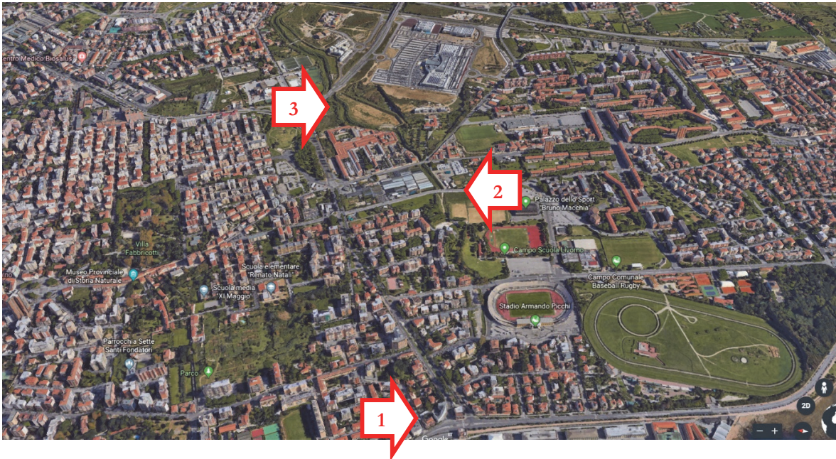
Figure 6: Top view of the area affected by the overflowing. (1) area of widest overflowing; (2) starting point where the Rio Maggiore is silted up; (3) one of the four detention basins.
