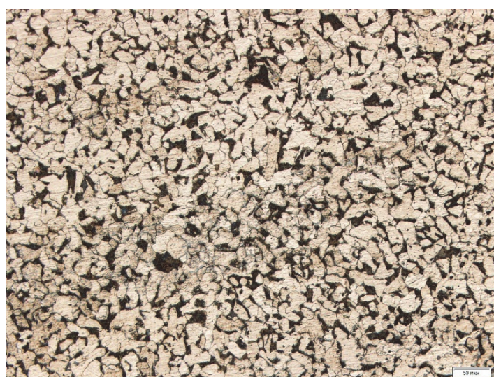
Figure 1: The microstructure of the carbon steel C1010.
