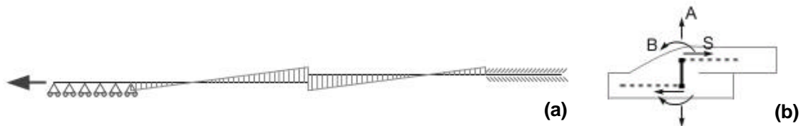
Figure 8. Structural model of the lap-joint: a) bending moments onto the clamped specimen; b) the lap-joint assimilated to a structural element.
