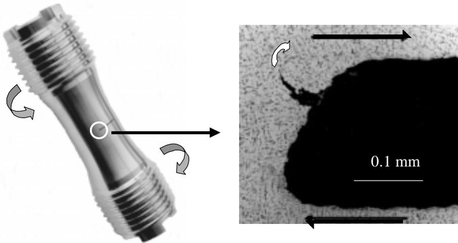
**Figure 5:** Crack propagation observed on the outer surface at the tip of the notch
