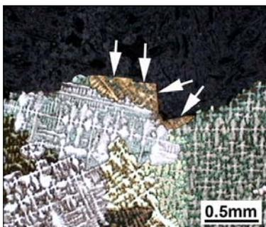
Figure 12. Crystallographic facets on the fracture profile. Axial section through the fracture surface.
