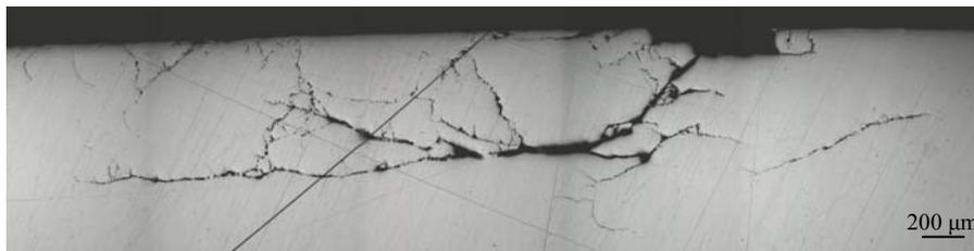
Figure 3. Specimen section in the spalling zone
