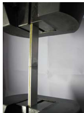
Figure 4. Tensile test apparatus of the spliced fiber metal laminate
