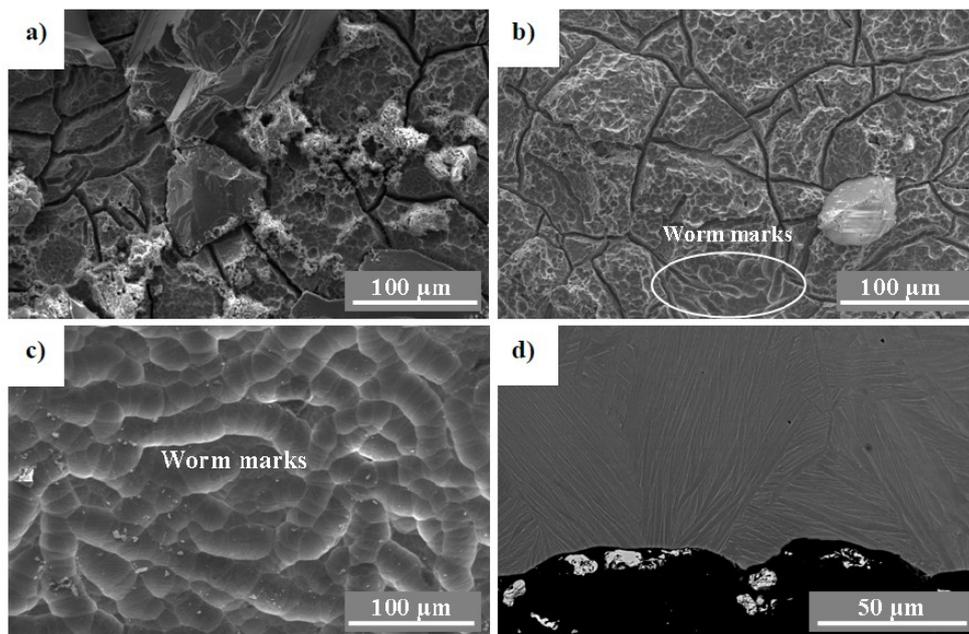
Figure 3: Pitting corrosion after: a) 20 min, b) 40 min, c) 60-70 min of pickling, and d) cross sectional SEM micrograph after 60-70 min of pickling
