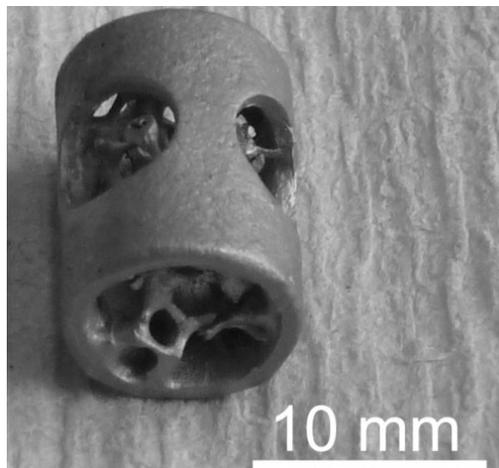
Figure 1: Open-cell titanium (Ti-6Al-7Nb) implants
