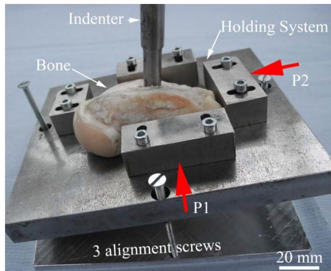
Figure 5: Push-out testing system used to analyse the ovine bone-implant interface
