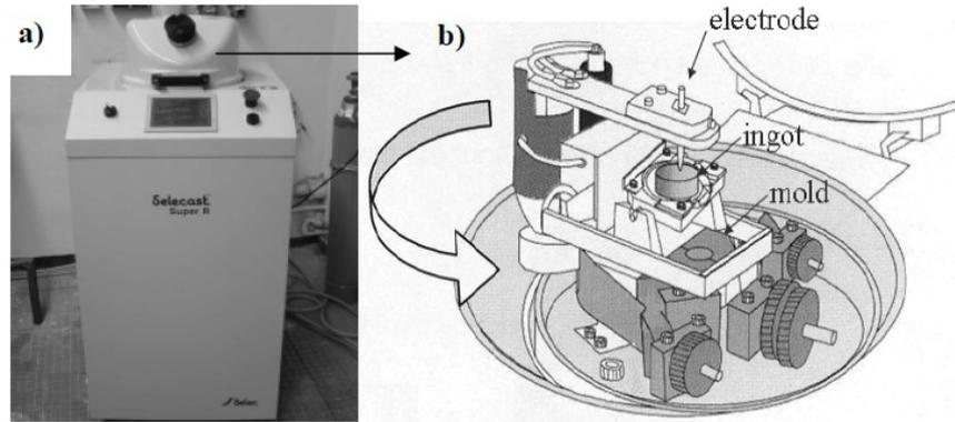
Figure 2: a) Centrifugal casting machine, b) schematic of the casting chamber
