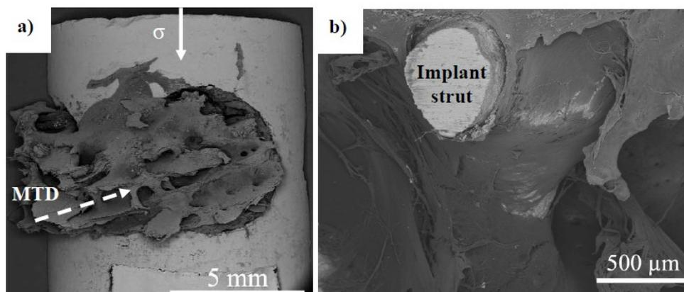
Figure 10: SEM micrograph of the ovine implants after the push-out test: a) external surface of the implant of the sheep #2, b) surface at the internal implant strut of the sheep #22
